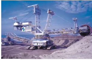
Excavator SchRs 1320/4x30 653 lubrication points
