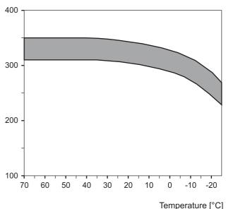
Pump's rotational speed depends on the operating temperature (only at EFP-1) Rotationalspeedofpumpmotor[min<sup>-1</sup>]
