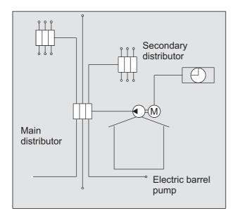
The lubricant of the electric barrel pump is directly delivered into the main progressive distributor, which has to supply the lubricant to the secondary progressive distributors in the right relation. The secondary distributors deliver the optimal lubrication quantity to the individual lube points.
