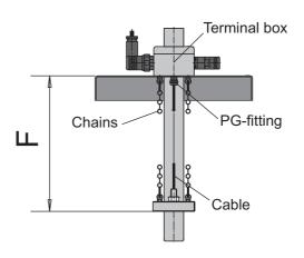
Dimension F must be smaller than dimension H, so that the pump does not prime air when being emptied.
