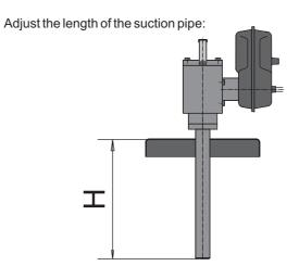
Dimension H should be smaller than dimension X, so that the pump pipe does not touch the reservoir ground.
