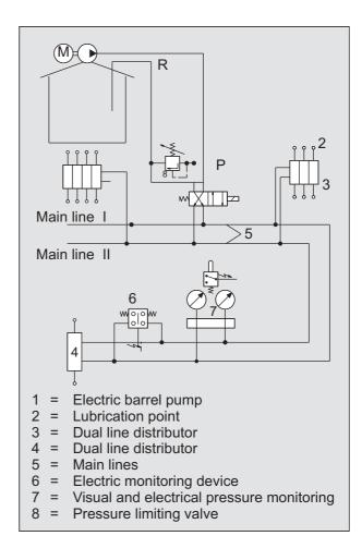
The dual line system is a system with two main lines, which can be pressurized via a valve alternately, and thus supply dual line distributors with lubricant.
